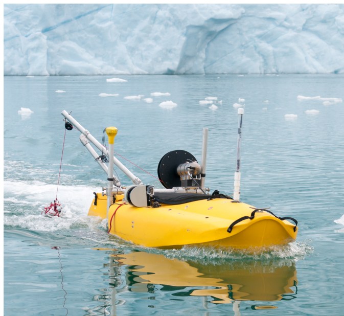
Fig. 1. A WHOI Jetyak returns to safety after collecting oceanographic data at the face of Sarqarliup Glacier in Greenland.
