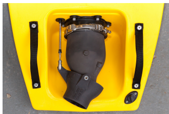
Fig. 4. A custom servo-driven control system utilizes full steering throw of the jet duct. Here, the duct is pictured as in a turn to port.
