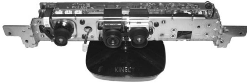
**Figure 1.** Kinect with external case removed showing the three primary sensors: IR structured light projector (left), RGB camera (center left), and IR detector (center right).
